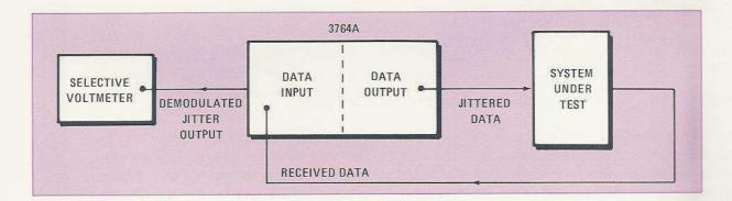
Totalized Jitter Hit Measurements - A Jitter Hit occurs when the peak-peak amplitude of received jitter exceeds a set threshold level. The number of jitter hits occurring during a gating period is counted. In addition, the number of seconds during a gating period in which a Jitter Hit occurred can be counted (Jitter Hit Seconds), as can the number of seconds in which no Jitter Hits occurred (Jitter Hit Free Seconds).
