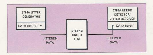
Jitter Transfer Function - The Jitter Transfer Function (i.e. Jitter Gain) is an indication of the accumulated jitter introduced when systems are cascaded. This must be controlled if data errors due to timing jitter are to be avoided. A system's Jitter Transfer Function can be expressed as:
