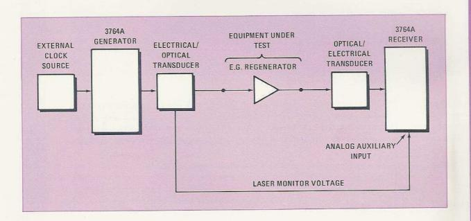
The 3764A's binary interface can operate over the range 1 kbit/s to 170 Mbit/s. This allows error measurements to be performed at the line rates of many digital transmission systems (e.g. 139 Mbit/s coded in 5B6B format gives a line rate of 167 Mbit/s). The value of the laser voltage can also be correlated with the measurement results and information from the built-in clock.
