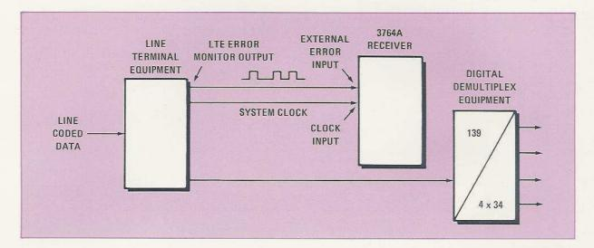
The 3764A's external error input allows errors detected by other equipment to be fully analyzed. This includes outputs from code and parity error detectors, where the error monitor equipment outputs its error information using the format one pulse per error.
