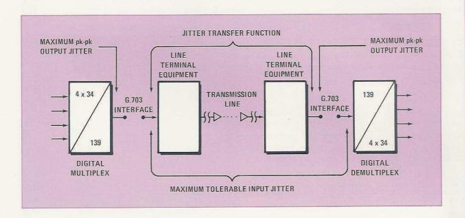
Maximum pk-pk Output Jitter — This is a measure of a system under test's inherent timing jitter. No input jitter is applied to the system while this measurement is made.
