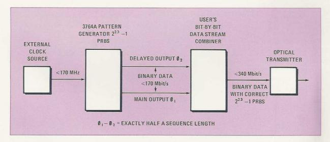
Recent advances in fibre optic technology have enabled submarine cable designers to consider using optical fibre as their transmission medium. Several systems have been proposed which involve multiplexing two 139 Mbit/s data streams. In the example shown, the 3764A's binary data streams are combined enabling an optical fibre system to be stimulated up to a line-rate of 340 Mbit/s. This removes the need for a separate high-cost high-speed signal generator.
