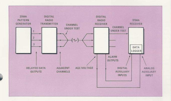
In this application the built-in data logger is very useful. The 3764A has eight auxiliary inputs (one analog and seven digital) which permit event recording, e.g. alarm conditions, along with measurement results. This data is logged along with information from the instrument's real-time clock. Consequently, a very effective low-cost solution to long term testing requirements is provided.
