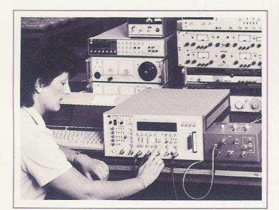
occur over the test period and these are subsequently correlated with other relevant data in a computer. This can identify failure-patterns and equipment weaknesses before they cause warranty problems.
