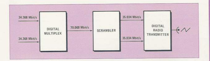
Any non-standard bit-rate between 1 Mbit/s and 170 Mbit/s can be provided at the binary interface by employing the 3764A's special option frequency, F2. Another typical example would be 140.434 Mbit/s which is used in a number of 11 GHz digital radios. This feature is useful in the manufacture and production test of digital radio systems.
